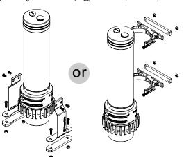
Attach fittings onto the pump and reservoir
