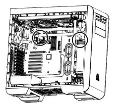
Connect the tubing and check all the fittings are sealed. The loop order: Pump Outlet > Radiator
