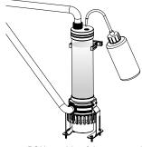
Place your PSU outside of the case and attach it to the pumps 4pin molex connector, turn on the power of PSU and make the rest of the system fills up.
